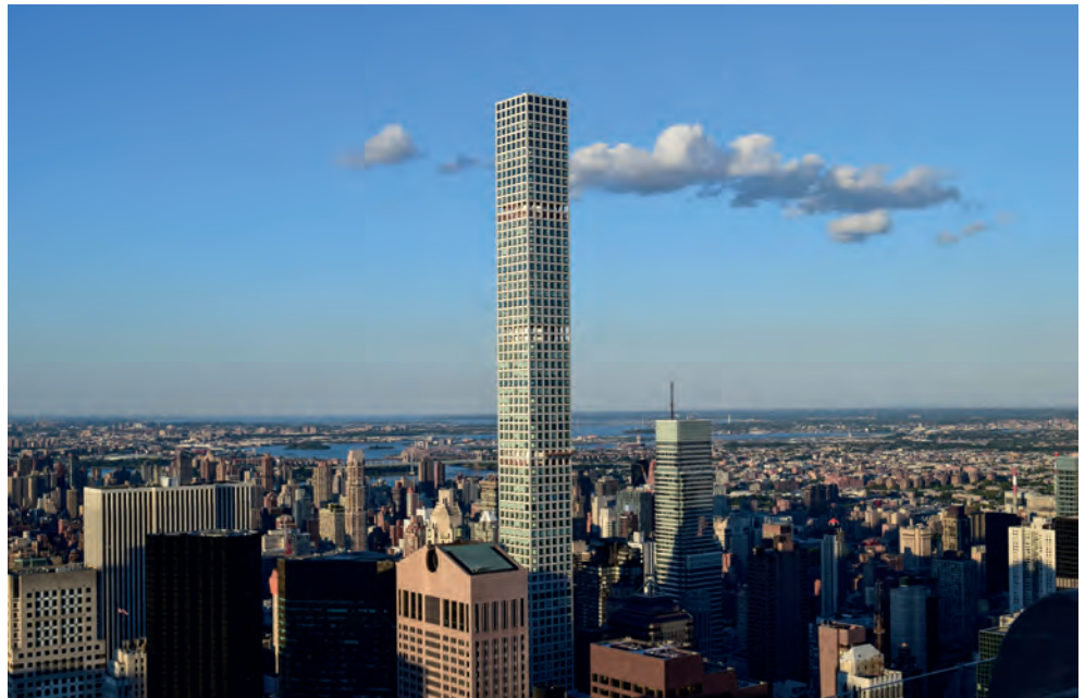
Above: At the super-skinny 432 Park Avenue in New York, a 111MPa mix enabled a height-to-width ratio of 15:1 Right: 100MPa concrete was used for the core of One World Trade Center
